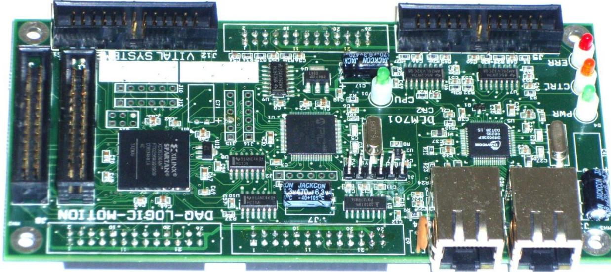
The HiCON is an Ethernet based controller for motion control, data acquisition, and general PID control system applications. Utilizing the latest Microchip technology, the HiCON offers a comprehensive set of features for your demanding applications.
