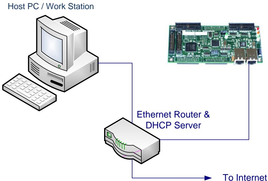
The figure above shows a basic setup using a router on your network. Connect the Ethernet cable from the J3 or J4 Ethernet port of the HiCON to the DHCP server/Router. Connect another Ethernet cable from the DHCP Server/Router to the PC. The DHCP server dynamically assigns IP address both to the PC as well as to the HiCON, and therefore completes the network setup without requiring any intervention from the user.
