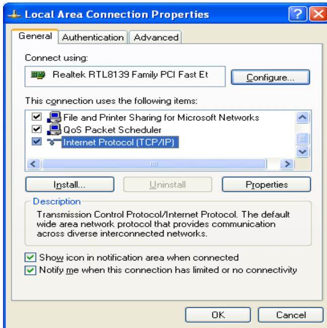
4. Click on the 'Properties' button and make the settings in your PC similar to the one shown in the figure below. After settings are done, click 'OK' button to finish the setup
